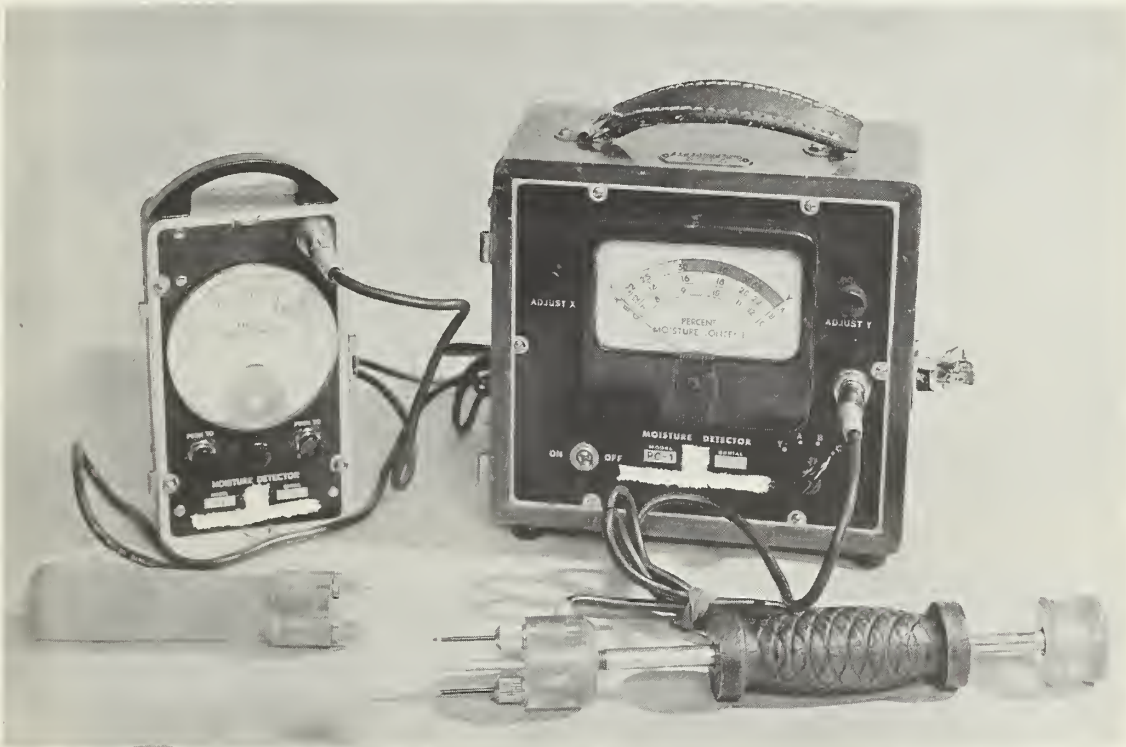
Figure 9. --Two sizes of resistance-type moisture meters showing needlepoint electrodes (left) and long, insulated electrodes (right).
